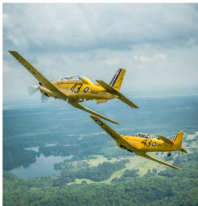
Two 'High Flight' Harvards, a wartime one and the modern Raytheon CT-156 Harvard II turboprop trainer both in BCATP colours
