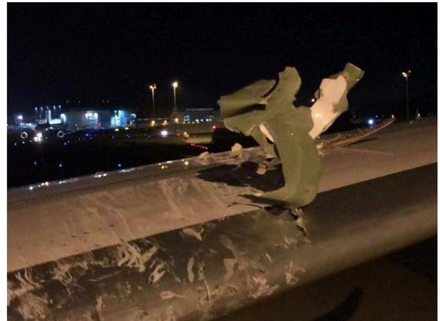
The TSIB found that the ATC staffer in charge of the 787, who was in training, made a number of mistakes, which led 9V-OJA to turn left on the wrong taxiway, where the collision occurred. It was found that the 787's left wing suffered damage which included the delamination and scuffing of multiple composite panels; multiple bent and abraded skin panels; cracked wing tip light lenses and severed static discharger wicks.
